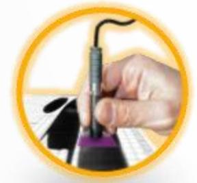
Thickness measurement over additional calibration film
